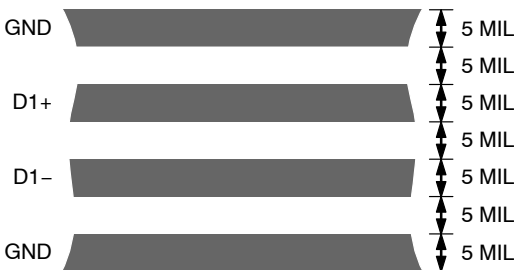
Figure 17. Arrangement of Signal Tracks
